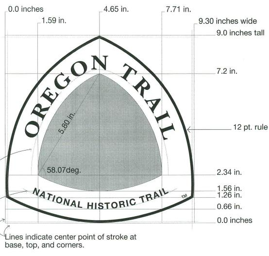
Lettering is based on parabola baselines identical to existing markers. For new designs use electronic template for generic logo.
